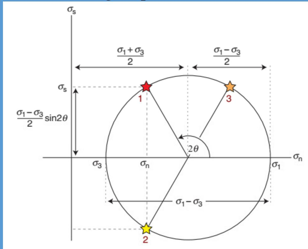
The Mohr circle  $\theta$  is the angle between the largest stress and a given plane.
