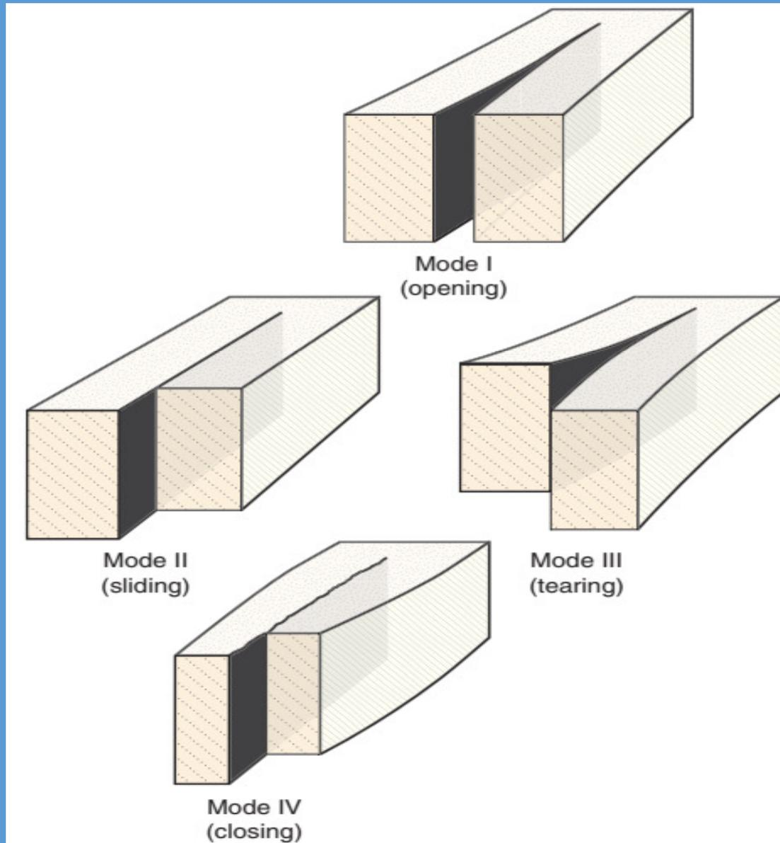
**Mode I** is the opening (extension) mode where displacement is perpendicular to the walls of the crack.
